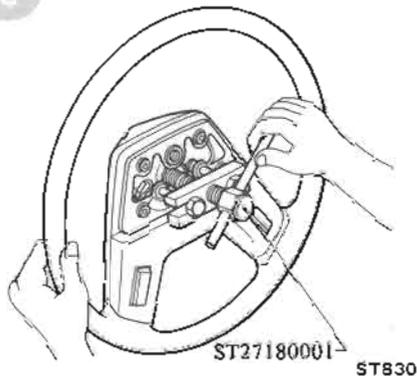
Fig. ST-2 Removing Steering Wheel
