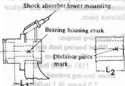
Fig. RA-17 Marking Position of Bearing Housing and Distance Piece
