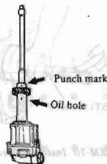
Fig. EM-79 Setting Distributor Driving Spindle
