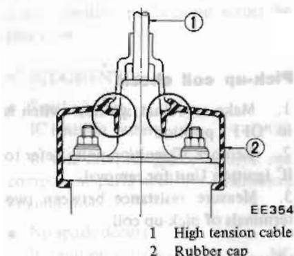
**Fig. EE-71 Correct Installation of High Tension Cable**
