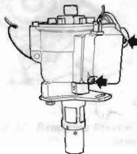
Fig. EE-64 Removing IC Ignition Unit
