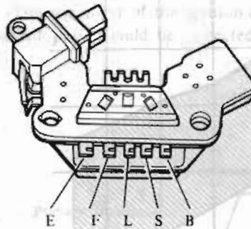
Fig. EE-48 IC Voltage Regulator
