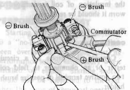
Fig. EE-8 Removing Brush
