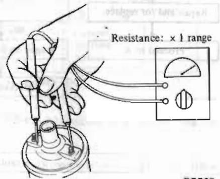
Fig. EE-69 Checking Ignition Coil Assembly
