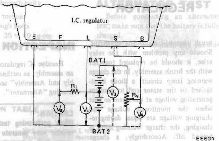
Fig. EE-50 Testing Regulator (1)
