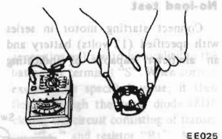
Fig. EE-17 Testing Brush for Ground
