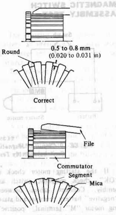
Fig. EE-13 Undercutting Insulating Mica
