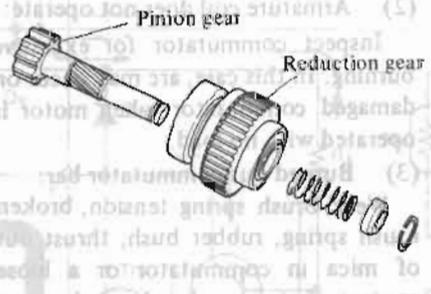
Fig. EE-16 Pinion and Reduction Gear Overrunning Clutch
