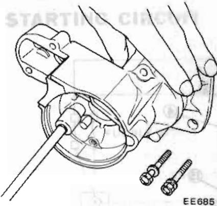
Fig. EE-9 Removing Center Housing
