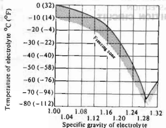
Fig. EE-4 Freezing Point of Electrolyte
