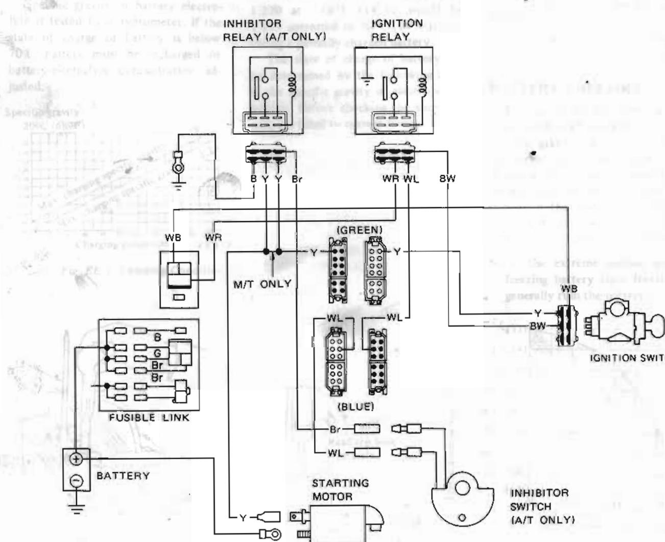
Fig. EE-5 Circuit Diagram of Starting System
