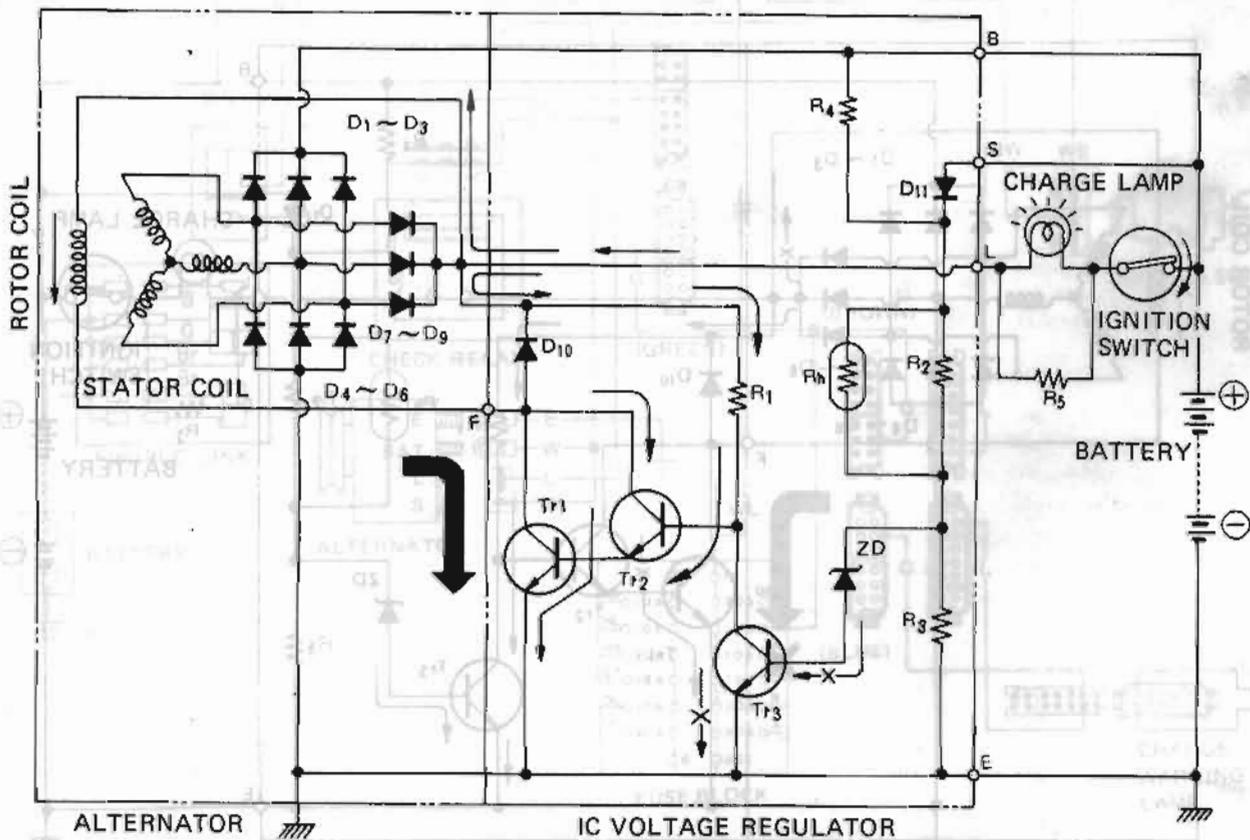
Fig. EE-21 Simplified Charging Circuit (Initial excitation current)
