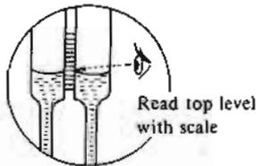
Fig. EE-2 Checking Specific Gravity
