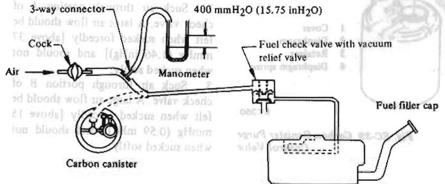
Fig. EC-37 Checking Evaporative Emission Control System
