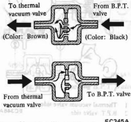
Fig. EC-16 Operation of Vacuum Delay Valve
