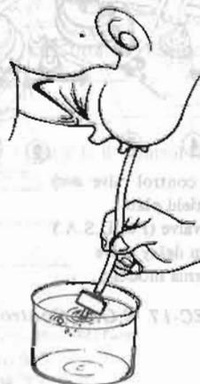
Fig. EC-24 Checking Vacuum Delay Valve
