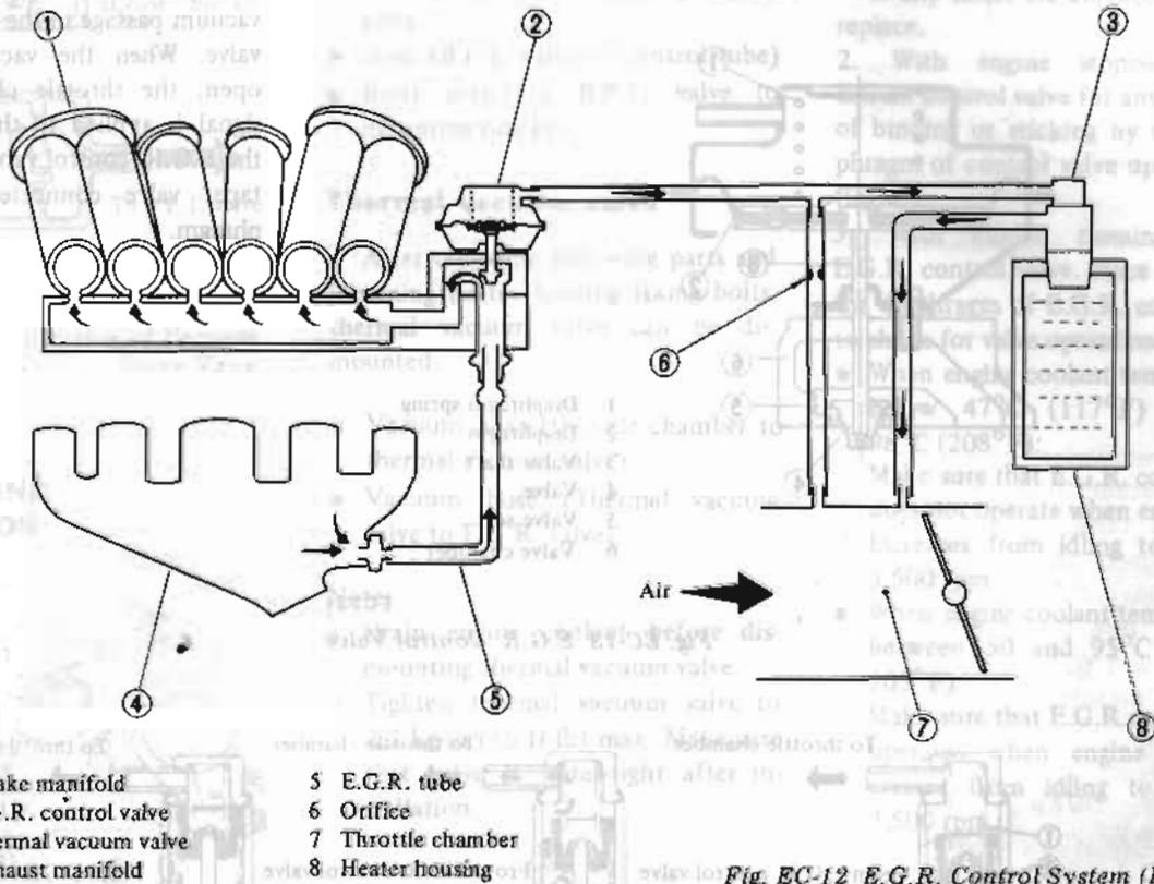
Fig. EC-12 E.G.R. Control System (For Canada)
