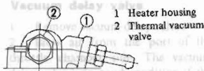
Fig. EC-18 Removing Thermal Vacuum Valve
