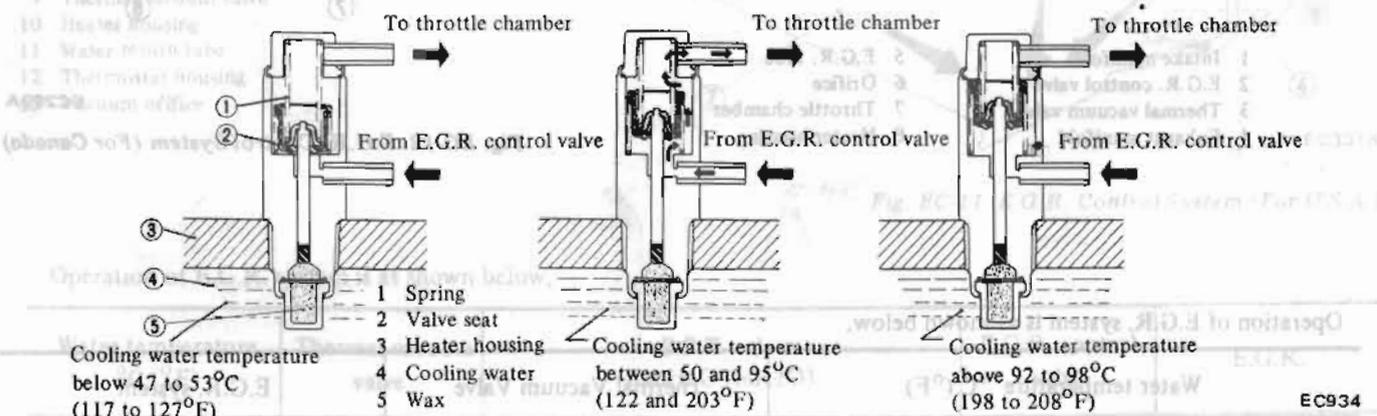
Fig. EC-14 Thermal Vacuum Valve
