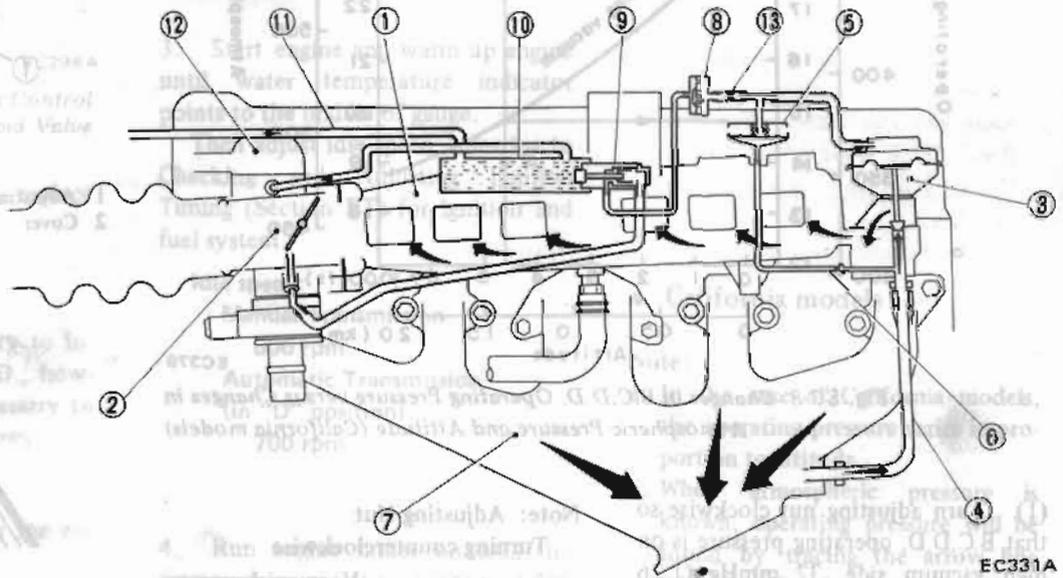
Fig. EC-11 E.G.R. Control System (For U.S.A.)
