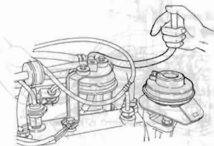
Fig. EC-21 Checking B.P.T. Valve
