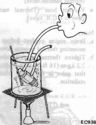
Fig. EC-22 Checking Thermal Vacuum Valve
