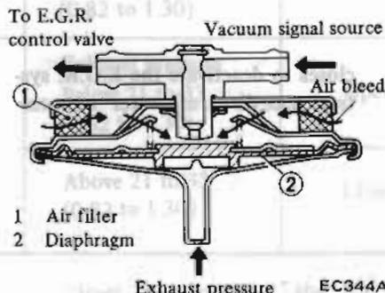
Fig. EC-15 B.P.T. Valve
