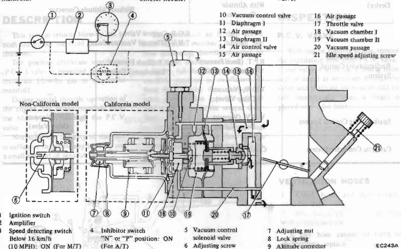
Fig. EC-2 Schematic Drawing of B.C.D.D.
