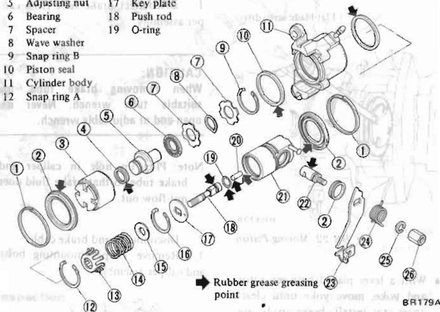
Fig. BR-28 Assembling Piston
