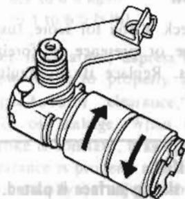
Fig. BR-27 Disconnecting Inner and Outer Piston
