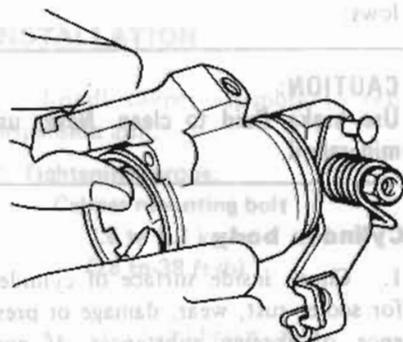
Fig. BR-26 Removing Piston
