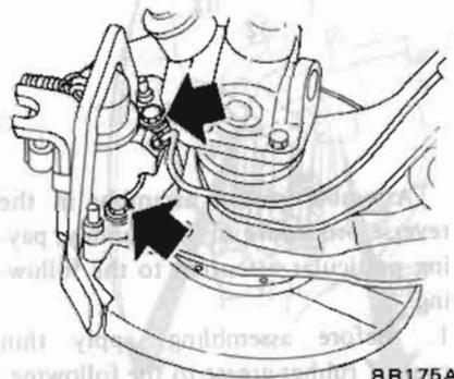
Fig. BR-24 Removing Caliper
