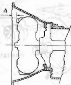
Fig. AT-25 Installing Torque Converter
