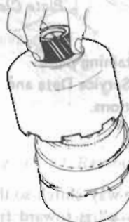
Fig. AT-47 Installing Connecting Shell
