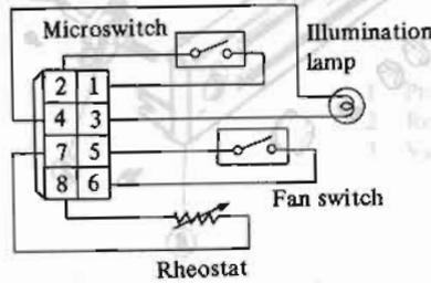
Fig. AC-45 Fan Switch and Microswitch
