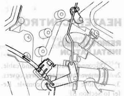
Fig. AC-47 Adjusting Temperature Control Lever
