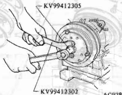
Fig. AC-57 Removing Clutch Hub Nut
