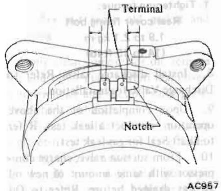
Fig. AC-91 Placing Clutch Terminal in Cut Portion of Shell
