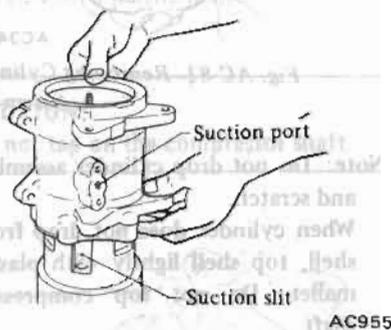
Fig. AC-89 Installing Shell
