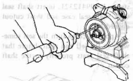
Fig. AC-62 Loosening Coil Mounting Screw
