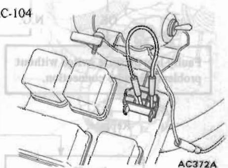
Fig. AC-104 Checking Cooler Relay
