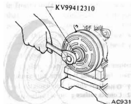
Fig. AC-60 Removing Lock Nut
