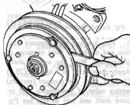
Fig. AC-64 Checking Clutch Hub-to-Pulley Clearance
